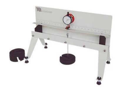
**Spring Test Apparatus Test Equipment - TQ- SM110**
